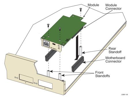
Figure C-5 Installing the Fast Ethernet Interface Module
